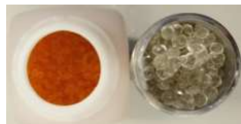
Figure 10 new desiccant orange (left), used desiccant transparent (right)
